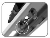
3. Secure cleat to the mounting surface using 1 or 2 X M10 bolts, adding a washing and nut on both sides.
